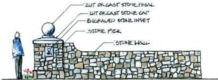
WALL UNSCROLLED ELEVATION ENTRANCE PIER AND WALL
